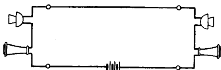
FIG. 1. A simple series telephone circuit.
