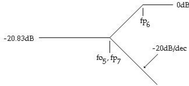
Fig.8 Bode plot of the treble response
