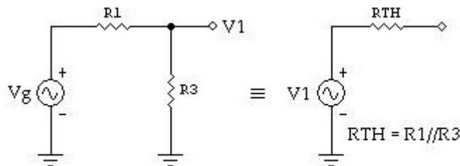
Fig.7 Thevenin equivalent for  $V_g$ ,  $R_1$  and  $R_3$
