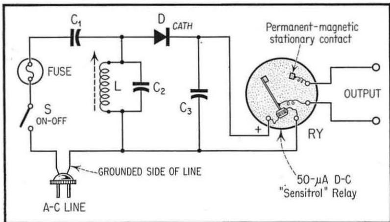
Fig. 3. Diode-Type Wired-Radio Receiver.
