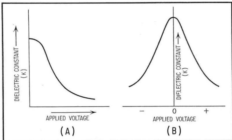
Fig. 1. Variation of Dielectric Constant with Applied Voltage.
