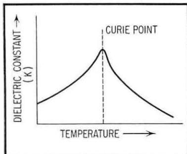
Fig. 2. Variation of Dielectric Constant with Temperature.
