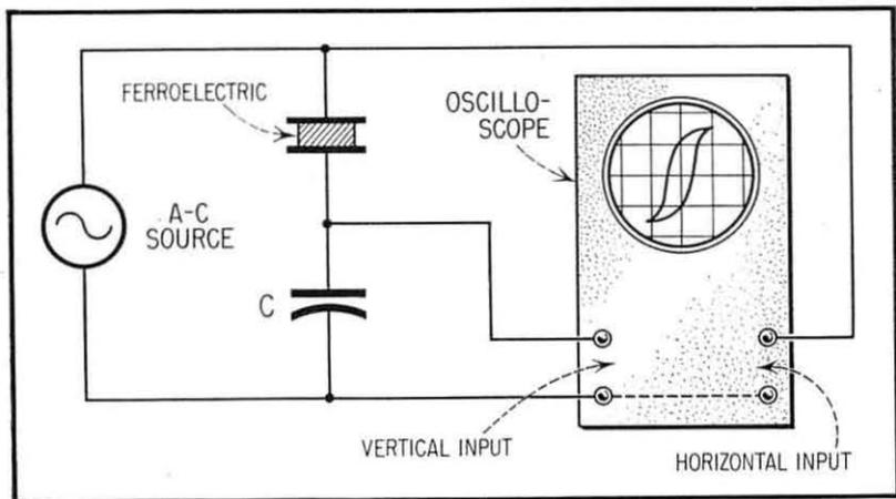
Fig. 3. Setup for Checking Ferroelectric Hysteresis.
